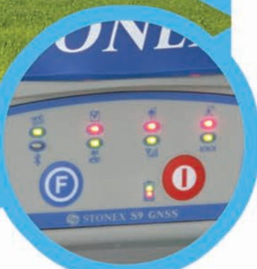
New front panel with indicators led for individual functions to indicate the status of receiver
